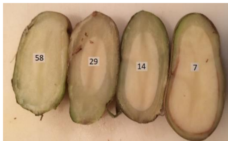
Figure 1: Time, measured as the number of 'whistles' required for complete gelation of potato starch
