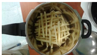
Figure 2: Arrangement of cut potatoes in pressure cooker before pressure reduction.
