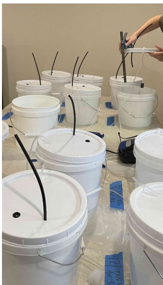
Figure A2. Sample access port preparation
