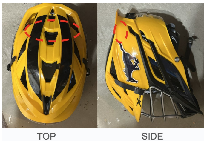
Figure 7. Location of Sensor in Helmet. The red dashed lines indicate the location of the sensor in the helmet.
