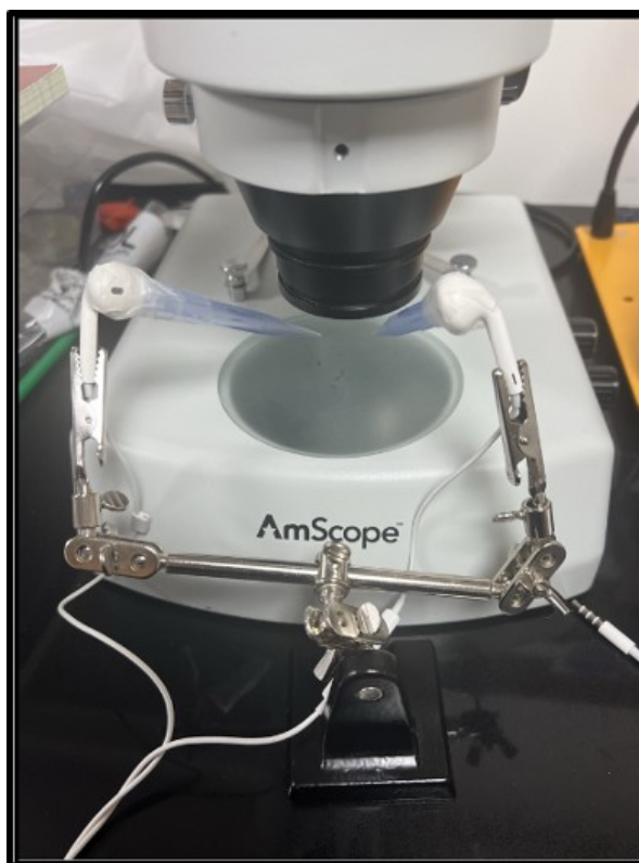
Figure 1. Speaker system that emitted frequencies with precise accuracy when directed at a worm, which allowed for the angle and distance from the plate to be adjusted.
