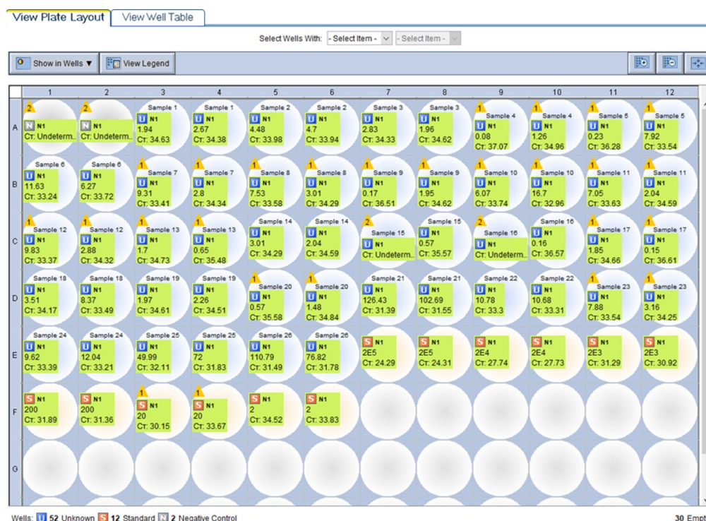
Figure 4. RT-qPCR Detection of SARS-CoV-2 RNA from 12 Environmental Samples. This was the second RT-qPCR assay by using SARS-CoV-2 RUO qPCR Primer & Probe Kit N1 primers/probe based on Lu et al (20).
