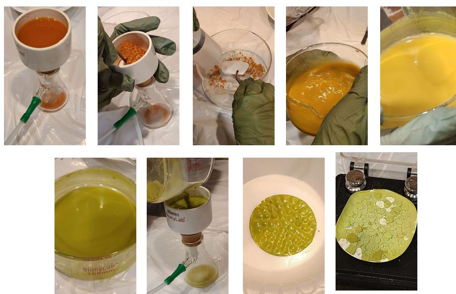
Figure 3. Progression of CuCl extraction after electrolysis, and purification. Top left to bottom right: Filtration of precipitate mixture, Precipitates separated from water, Before HCl reaction (0 minutes), During HCl reaction (10 minutes), During HCl reaction (20 minutes), During HCl reaction (40 minutes), Filtration of product, Product on filter before drying, Dried product on filter.
