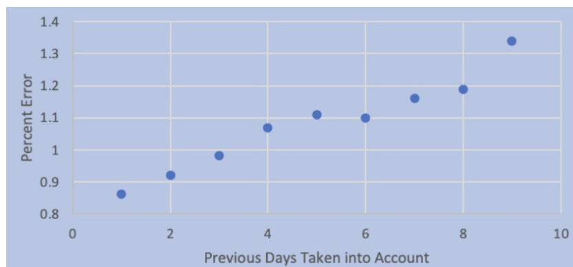
Figure 8. Average percent error versus number of previous days the data was drawn from
