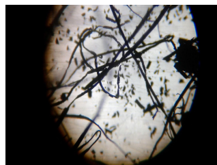
Figure 2: Steel Wool after combustion
