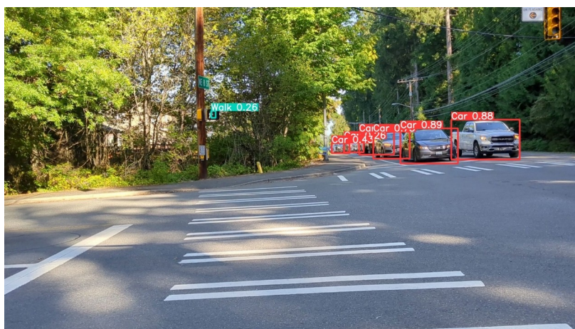
Figure 6. shows the result of running the object detection model on Figure 5. The model was able to detect the cars and the walk sign on the pedestrian traffic light.
