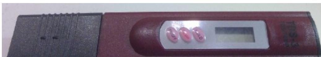
Figure 5: Digital turbidity meter. Model is a TDS-3, made by HM digital, Vista, CA.
