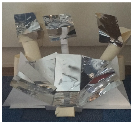
Figure 2: The solar reflector used in the experiment. Water samples, in a clear glass bottle, were placed on the Mylar square in the center foreground of the image
