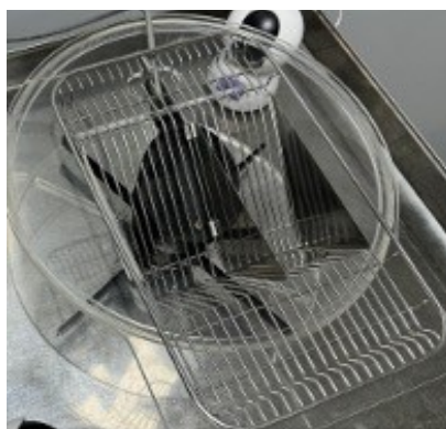
Figure 1. Rotor Cage. A custom-made rotor cage was used to effectively sleep deprive the mice without introducing additional psychological and physical stress that could confound results.
